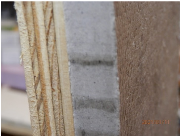
Cut using Festool showing minimal "curl"
