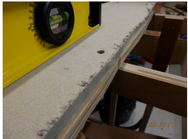
Cut with Bosch blade showing edge "curl"
