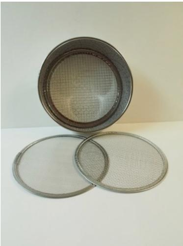
The grid sizes are: Fine – .065", Medium – .100", and Coarse – .250". These are the sizes used in the following example photos. It's important to note when looking at the photos that the .065" screen will pass up to .065" and anything smaller so if you're working in small scales you may want to source a
