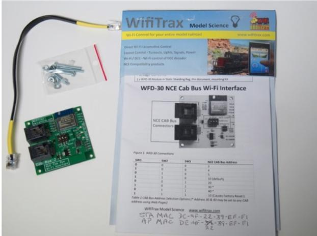
Reading the quick start pamphlet revealed that there wasn't much to do. I had already installed WiThrottle on my iPhone, so all that was left was connecting the NCE cab bus cable and selecting the WFD-30's Wi-Fi network on the phone.
