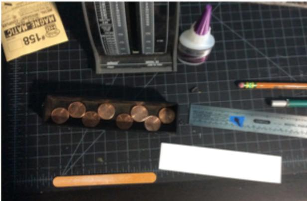
The first step was to glue the eight pennies onto the gondola's original floor with gap-filling medium CA. Then, using .060 styrene, I scored and snapped a new floor to fit over the pennies. Using an emery board, I sanded the floor to fit, and then I glued it into place with the CA. After the CA dried, I brush painted the interior of the gondola with
